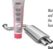
Water-based mounting paste with heat-resistant filler. It has been developed especially for the assembly of exhaust systems in automotive and general industrial applications. It has a heat-drying mechanism. After applied, the engine is started and the drying is accelerated with the exhaust heat. It provides excellent sealing against carbon monoxide and other hazardous exhaust vapors after being completely hardened. Heat Resistance: 1000°C
